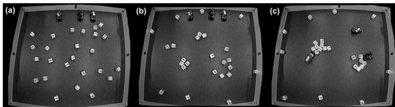
Figure B1. Example of clustering behavior by didabots. (a) Initially, the cubes are randomly distributed over the arena. (b) Over time, clusters begin to form. (c) By the end of the experiment, there are only two large clusters, with the remainder of cubes aligned along the walls of the arena. Reproduced with the permission of Rolf Pfeifer and the Artificial Intelligence Laboratory, University of Zurich.
