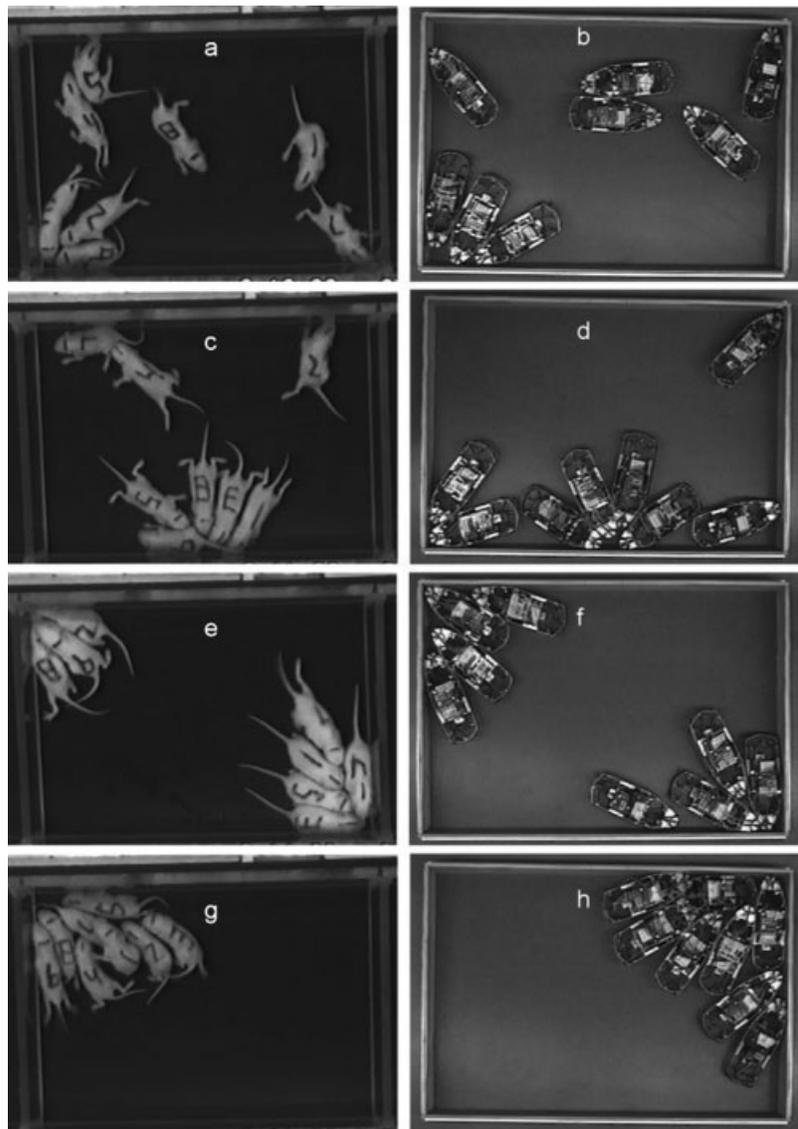
Figure B2. Rat pups and robotic rats forming aggregation patterns. (a) 7-day-old pups and (b) robots shortly after they are released or started in the arena, (c) 7-day-old pups and (d) robots forming a subgroup; (e) 10-day-old pups and (f) robots forming two subgroups in opposite corners; (g) 7-day-old pups and (h) robots forming a group in a single corner. Reproduced with permission from Wiley-Liss Publishers.
